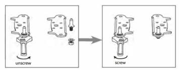
6. Refit the bracket fitting the bottom hinge pin. Replace both adjustable
