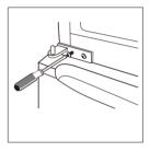
11. Place the upper door back on. Ensure the door is aligned horizontally and vertically so that the seal are closed on all sides before finally tightening the top hinge. Then inert the top hinge and screw it to the top of unit and then fix hinge cover (in accessary bag) by screw.
