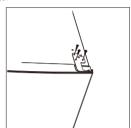
2. Remove the pin with a screwdriver and flip the hinge bracket. Then refit the pin to hinge bracket.
