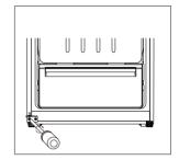
10. Make the middle hinge reverse the direction 180°C, then transfer it to the left property position. Make the middle hinge pin in the upper hole of the lower door, then tight the bolts.
