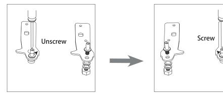
7.Refit the bottom hinge. Replace the adjustable feet.
