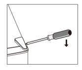
2.Undo the screws.Then remove the hinge bracket.
