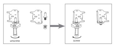
6. Refit the bracket fitting the bottom hinge pin. Replace both adjustable feet.
