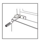
7. Install the upper door, fix the upper door hinge onto the cabinet .
