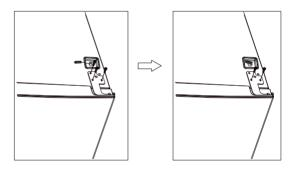
2. Unscrew from the middle hinge by cross screwdriver, then take off the lower door.
