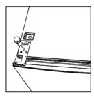
8. Take left hinge cover from accessary bag and install it with top hinge. Then install hole cover at right side.
