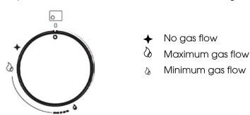
All operating positions must be set between the maximum and minimum flow settings, and never between the maximum setting and the closed position.
