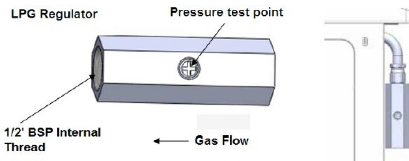
When the installation is complete, always check that all the unions are absolutely tight using a soapy solution. Never use a flame to make this check.
