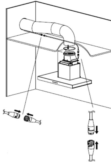
Note: You need to loosen the connecting wire before repair, follow the steps as below:
