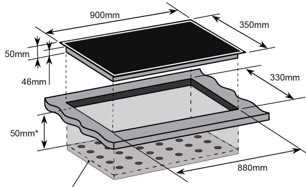
\* A thermal protection heat barrier **MUST BE** fitted 50mm from the base of the cooktop when access is possible via a cupboard or drawer. This thermal protection heat barrier should contain holes to improve ventilation as shown.
