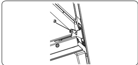
3. Close the door until it almost reaches the fully closed position and remove the door by pulling it towards you.
