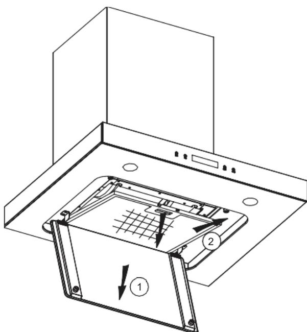
1. If the rangehood has a perimeter panel, then pull down to reveal the mesh filters, otherwise proceed directly to Step 2.
