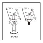
6. Refit the bracket fitting the bottom hinge pin. Replace both adjustable feet. Transfer the lower door to the property position.
