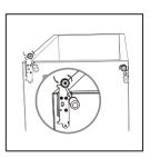
Unscrew right middle stopper with metal block from bottom of upper door. And then install left middle stopper and metal block in left side of bottom of upper door. (The same operation as for lower door.)
