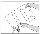
3-If there is lint accumulation in the funnel of the water tank, clean it under running water.
