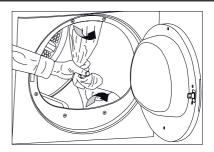
⚠Make sure that you have removed the transportation safety assembly (nylon+styrofoam pieces) before using the product for the first time. Do not leave any items inside the drum.
